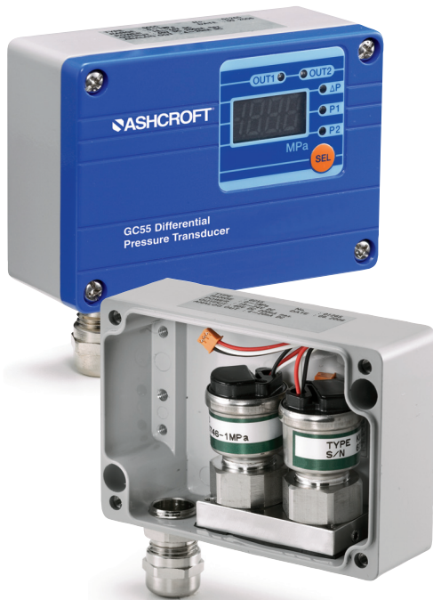
Two sensor DP design means three measurement variables in one device. Output, display and switch settings can be set in nearly ANY independent configuration to monitor, high pressure port (P1), low pressure (P2), differential (P1-P2).
